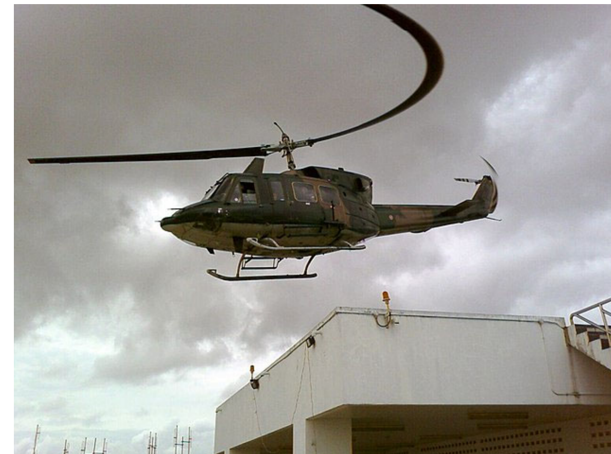
Disadvantage of CMOS: Rolling Shutter
