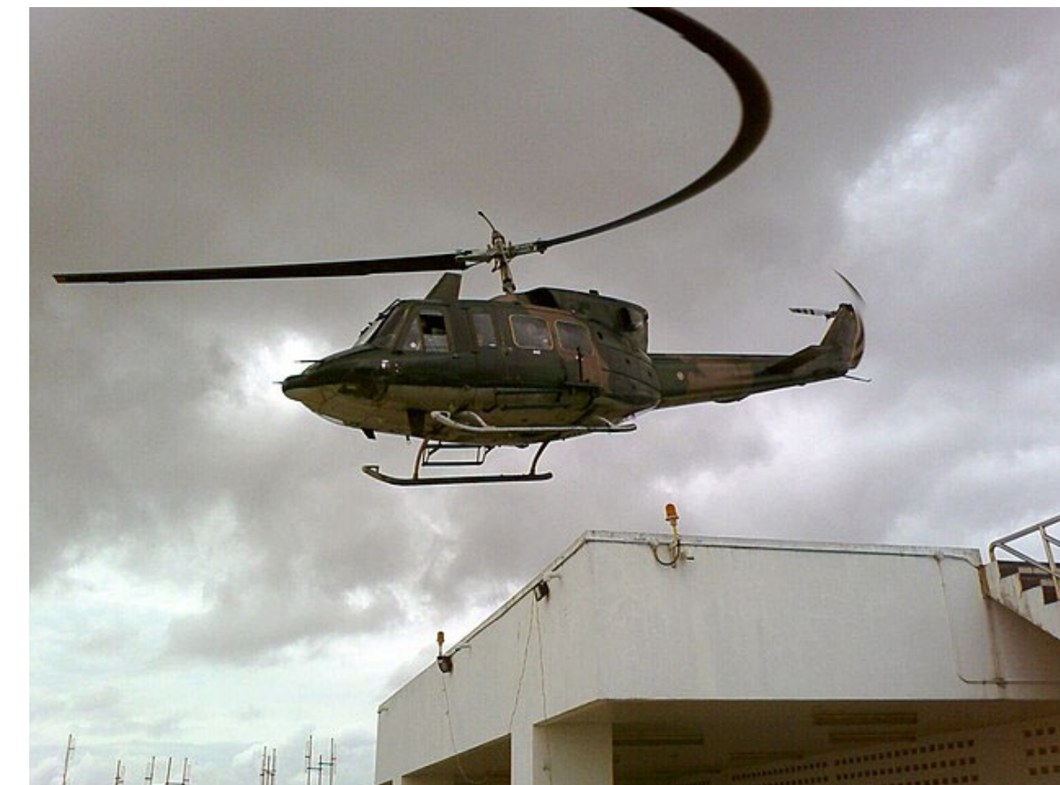
Disadvantage of CMOS: Rolling Shutter
